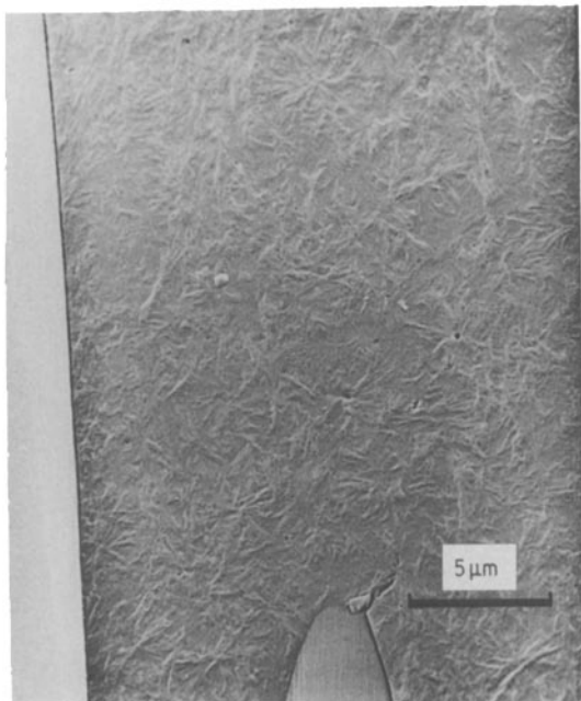
Figure 8 Scanning electron micrograph of etched longitudinal section of a laminate with abnormal orientation.
